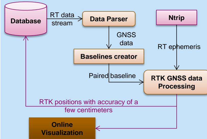
In the project X-Sense, a real time monitoring system has been developed based on wireless sensor network and RTK (Real Time Kinematic) GNSS positioning technique.
