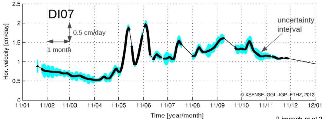
**Figure left:** Horizontal velocity for station DI07 (located on the rock glacier) obtained from static solution. There is a general increase of the velocity during the summer months. The peaks in May and June are due to snow-melt.
