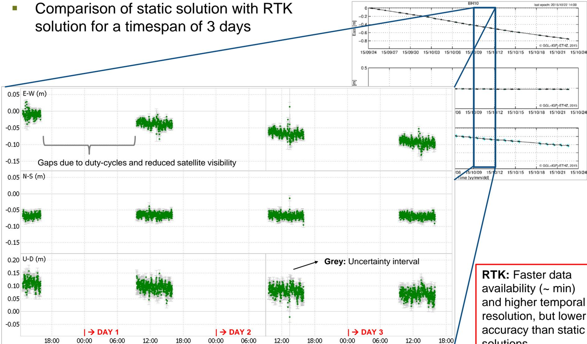
**RTK:** Faster data availability (~ min) and higher temporal resolution, but lower accuracy than static solutions
