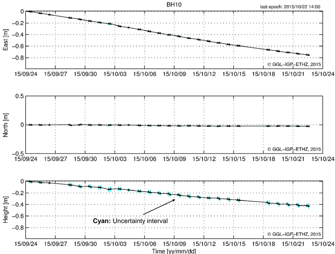
**Figure:** Change in East, North and Height coordinates of station BH10 wr.t. Sept 24. The triangles represent the static coordinate solutions. An almost linear movement of the station is visible in the east and the height component.
