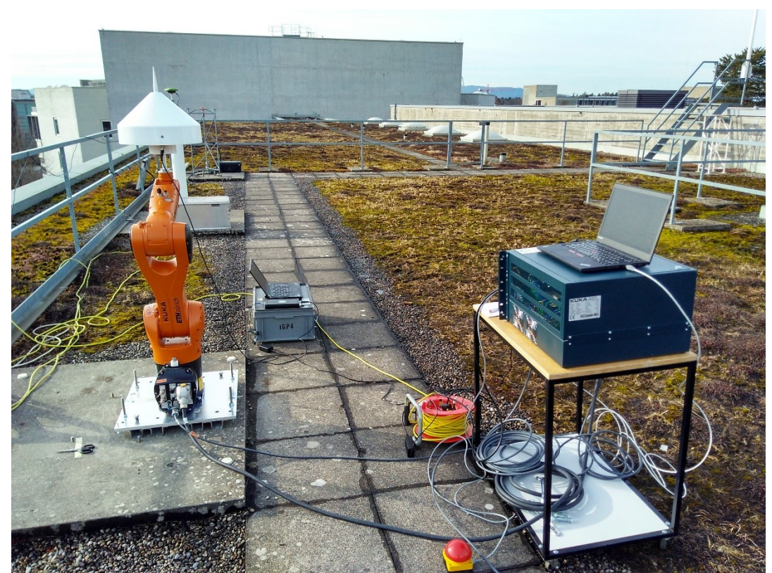
Figure: KUKA robot and GNSS equipment (LHS) and KUKA control unit (RHS)
